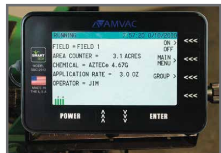
In-cab computerized controller for smart and easy precision application, monitoring and record keeping.
